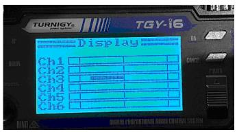
Stick fully down - trim full up - value above 'End Point' so display moves and so does the winch
