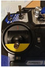
What about the fail safe function built in to prevent the radio operating unless the stick is all the way down? It turns out it doesn't have to be all the way down. By moving the stick in small increments up and attempting a restart of the radio the maximum position up of the stick can be found. I set the stop a little lower than this to ensure the radio starts reliably every time.
